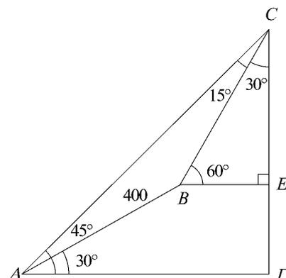
$$\triangle ACD \text{ 中, } \overline{CD} = \overline{AC} \sin 45^\circ = \frac{400 \cdot \sin 150^\circ \cdot \sin 45^\circ}{\sin 15^\circ} = \frac{400 \cdot \frac{1}{2} \cdot \frac{\sqrt{2}}{2}}{\frac{\sqrt{6}-\sqrt{2}}{4}} = 200(\sqrt{3}+1)$$
